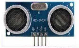
*Fig 1: Ultrasonic sensor*
