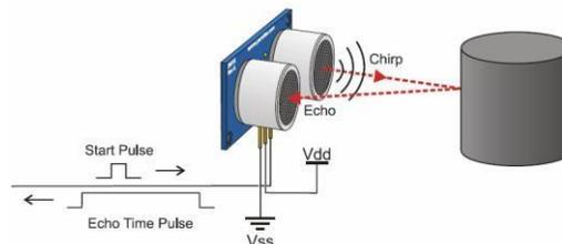
*Fig 3: Working of Ultrasonic sensor*
