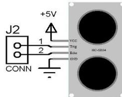
*Fig 2: Ultrasonic sensor circuit*
