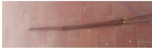
*Fig.7 Copper mesh wound upon heat pipe*
