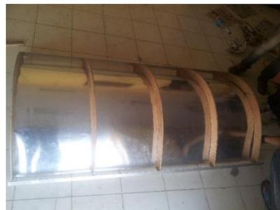
*Fig.4 Basic frame with aluminium sheet*
