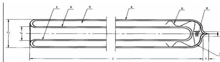
*Fig.8 Structure of all glass evacuated tube*
