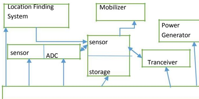
Figure 1: Major parts of a sensor node
