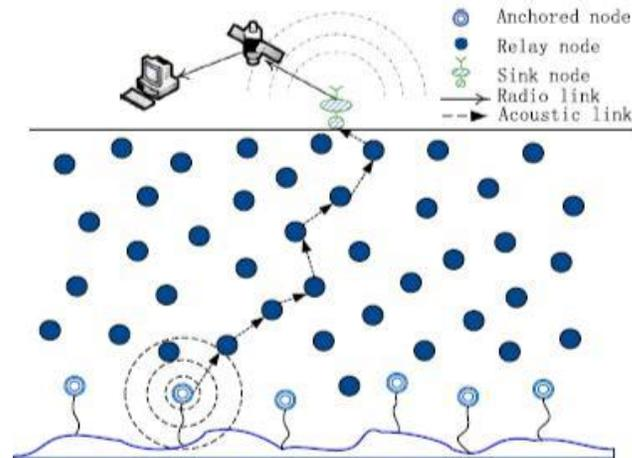
Figure 2: Architecture of the mobile UWSN
