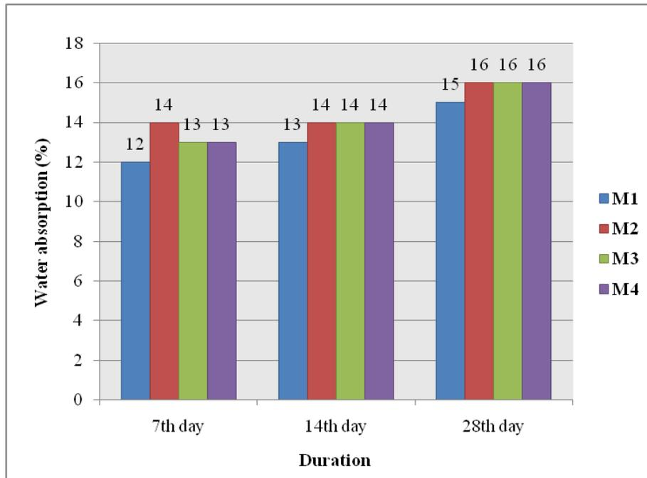
*Fig.6 - Water absorption of FaL-G Bricks*
