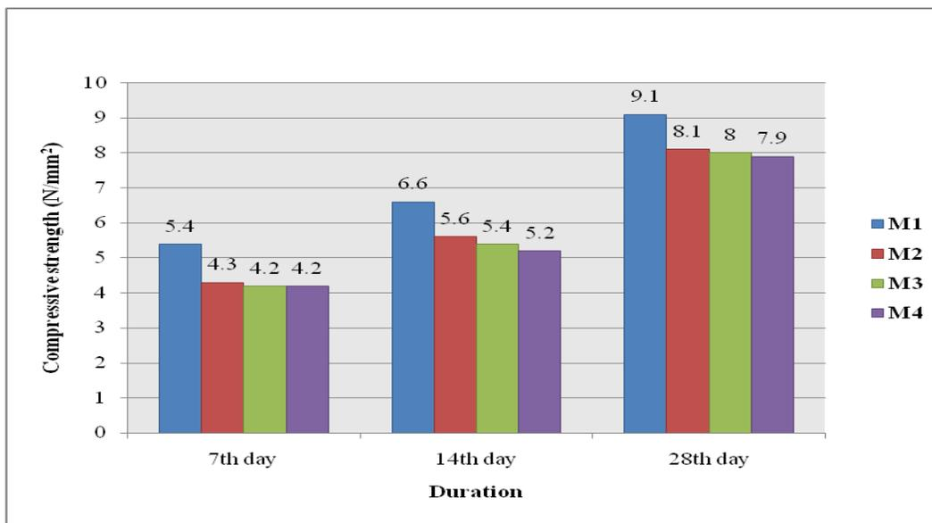
*Fig.4 – Compressive strength of FaL-G Bricks after sulphate intrusion*
