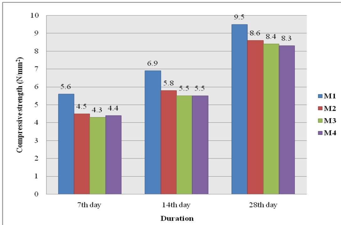
*Fig.2 – Compressive strength of FaL-G Bricks*
