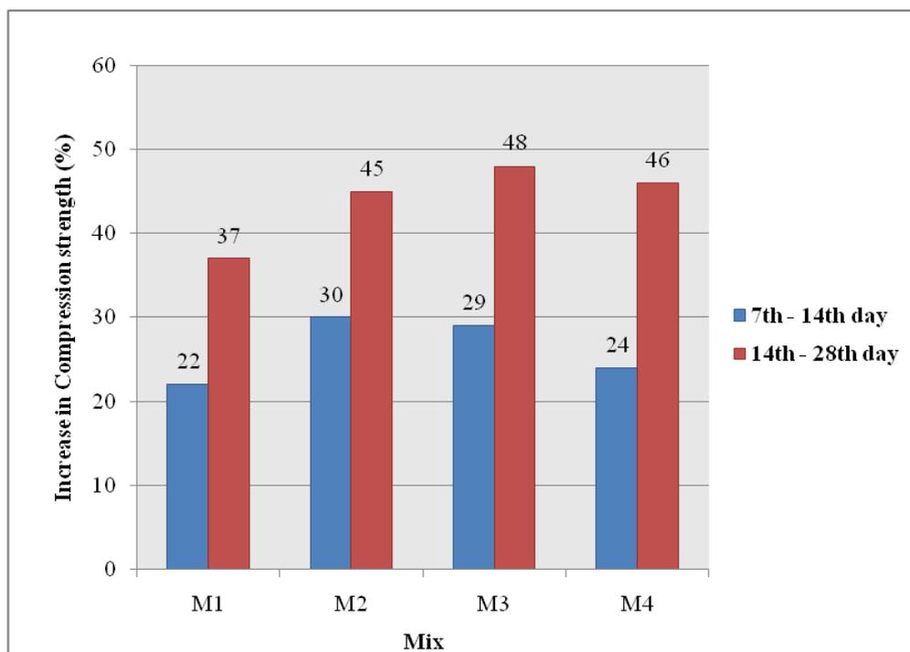
*Fig.5 Compressive strength comparison of FaL-G bricks with aging after sulphate intrusion*
