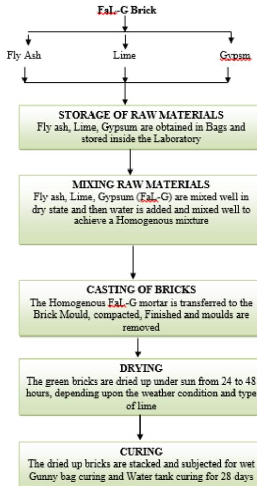
Fig 1 Schematic flow diagram
